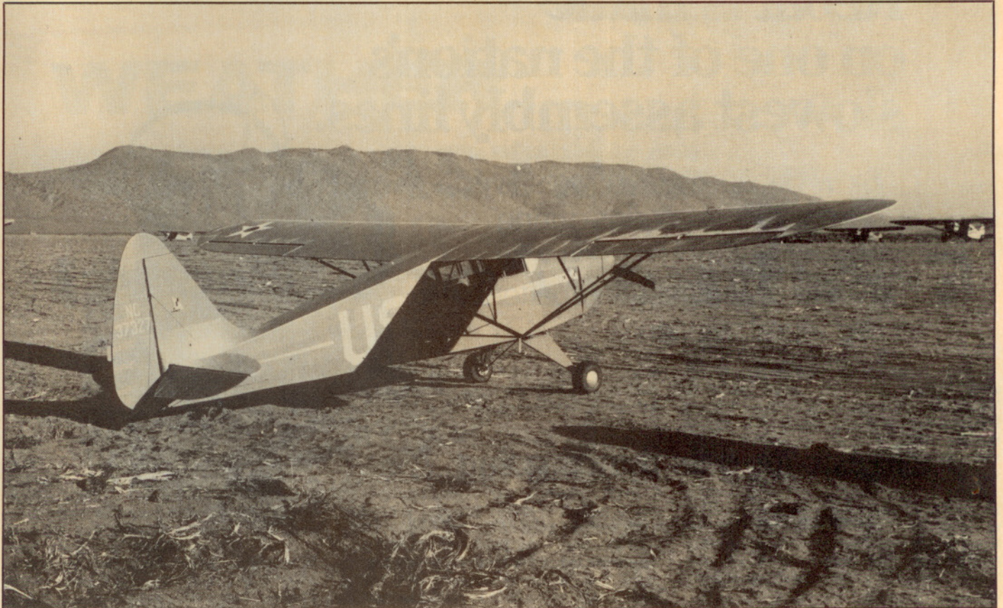
An Interstate S-1A-90F Cadet, photographed early in 1942. Note the considerably higher vertical tail and the balanced rudder. Civil planes in the West Coast Defense Zone had to carry the star insignia on the upper left and lower right wings, in addition to the letters "US" on the fuselage.
